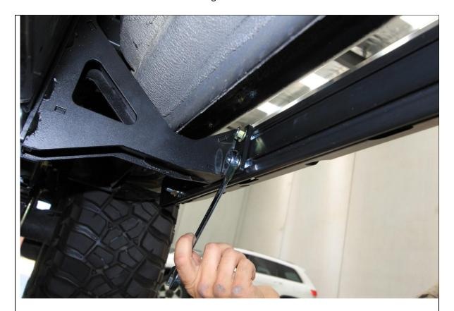
47. Tighten all mount to slider M10 flange nuts using 15mm spanner. A ratcheting spanner makes this process easier.
