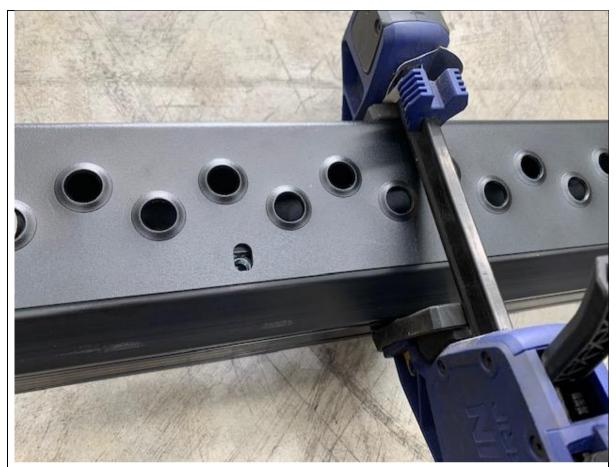
29. Using long tool feed nuts in to centre first and thread in with black M8 button head cap screws and washers
