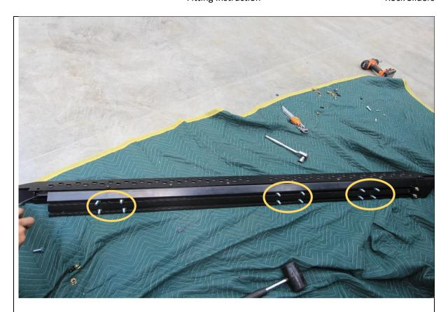
34. Slide the 12x M10x25 Hex bolts into the T slots on back side of extrusion. 6 bolts per slot.
